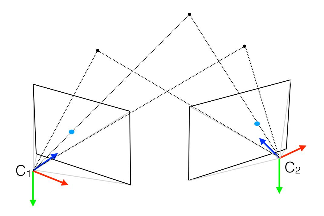
How to estimate the relative pose between the cameras from 3D-3D correspondences  $(p_{1,k}, p_{2,k})$  with k = 1, ..., N ?
