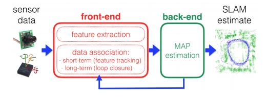
Figure 23.1: Front-end and back-end in a typical SLAM system.
