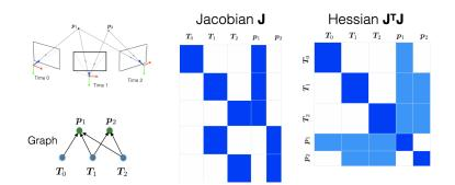
Figure 23.4: Bundle adjustment problem with 3 cameras and 2 landmarks. Sparsity patterns of the Jacobian and Hessian matrices.
